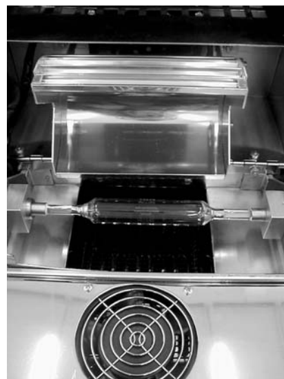
Accessibility to the optics is a critical feature of a UV-curing system.
