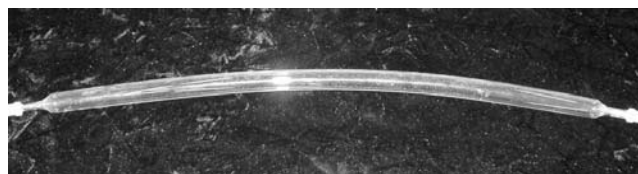
Bowing can occur with insufficient cooling of the lamp.
